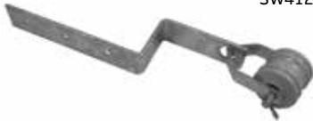
Add suffix "NI" if insulator is not required. Constructed of 3/16 in. x 1 1/2 in. steel, comes with catalog no. IB134 insulator. Three 3/8 in. round mtg. holes. All ferrous parts are hot dip galvanized.
