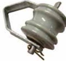
Add suffix "NI" if insulator is not required. Constructed of 3/16 in. x 1 1/2 in. steel, has 3/8 in. diam. pin and comes with catalog no. IB134 insulator. 1 1/8 in. round mtg. hole. All ferrous parts are hot dip galvanized.
