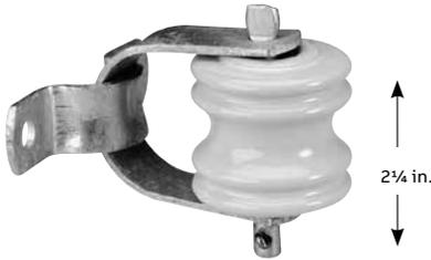
Add suffix "NI" if insulator is not required. Constructed of 3/8 in. x 1 in. curved mild steel, has 3/8 in. diam. swivel type pin, comes with catalog no. IB134 insulator, 2 mtg. holes 7/16 in. round. All ferrous parts are hot dip galvanized.
