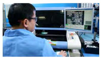
The AOI (automated optical inspection) machine added to our printed circuit board operation is one of the first of its kind in use in North America.
