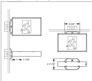
The **EZ2<sup>TM</sup> Canopy** allows the installer to make all of the electrical connections using both hands without having to juggle with the Exit Sign, making it our most contractor friendly product feature to date.
