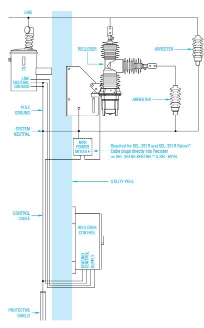
Arresters are recommended to provide protection against overvoltage conditions. When arresters are installed, they should be mounted on the supplied arrester brackets or as close to the recloser as practical.
