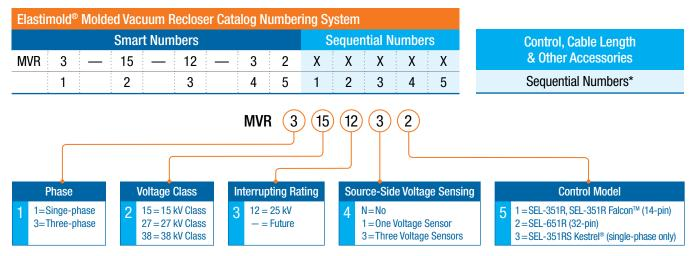
Single-phase reclosers function with the SEL-351RS Kestrel<sup>®</sup> control. Three-phase reclosers function with SEL-651R, SEL-351R, or SEL-351R Falcon<sup>™</sup> controls. The MVR Power Module must be specified when using a SEL-351R & SEL-351R Falcon controls.
