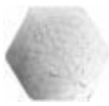
After air compression by the T&B Method, the cross section looks like this, 100% metal with virtually no air spaces.
