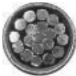
Before compression, a typical cross section of cable and connector consists of about 75% metal and 25% air.
