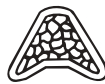
After Compression —the connector and conductor are formed into a solid mass.
