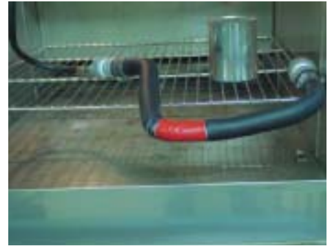
“Failure” repaired by tape under test.
