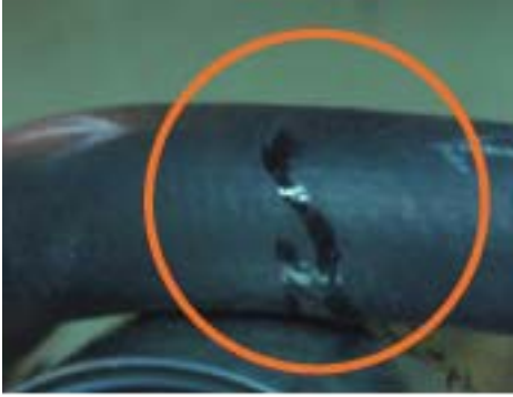
Close-up showing hole in rad hose.
